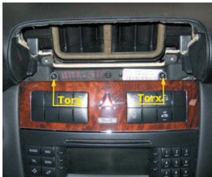
Remove ventilation shaft en remove 2x Torx 20. Then remove panel.
