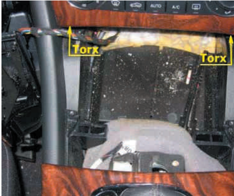
Remove 2x Torx 20 and use plastic wedge to remove panel.
