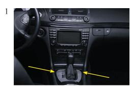
Remove the plastic trim around the gear lever. Remove the ashtray.
