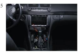
Place the replacement panel. Place the 2-Din metal bracket.
