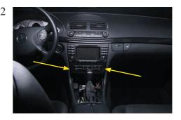
Remove the the screws and remove original storage bin/ CD changer.
