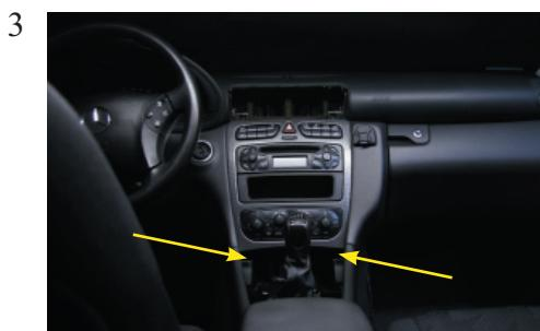
Pull the the dashboard towards you. At the location of the arrows there are clips which holds the dashboard in place.
