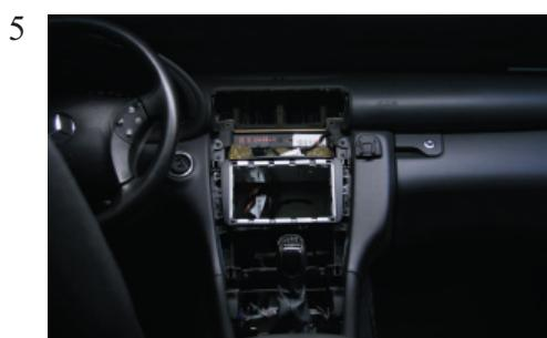
Place the replacement panel. Place the 2-Din metal bracket.
