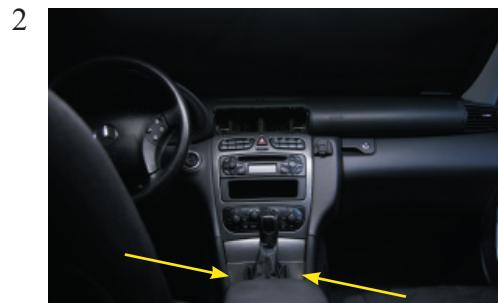
Remove the plastic trim around the gear lever. And remove the ashtray.
