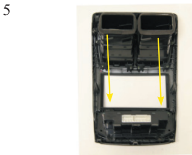
Mount the replacement panel at the back of the original dashboard panel.
