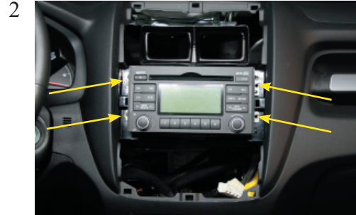
Remove the four Philips screws.
