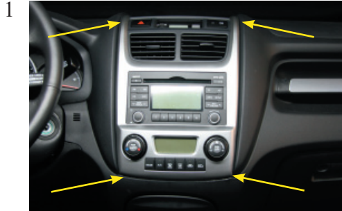
Remove the original dashboard panel using a plastic wedge.
