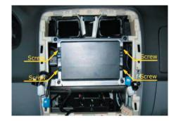
Remove 4 screws and remove the panel.
