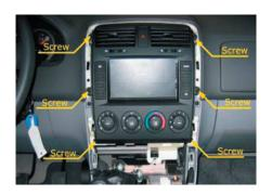
Remove 6 screws and use a plastic wedge to remove panel.
