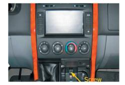
Remove 1 screw and use a plastic wedge to remove plastic rim.
