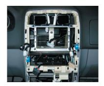
Place the head unit including mounting plates and supporting bracket.
