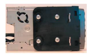
Remark: for motorized screen cut off 1,5 mm from the bottem of the ABS ring if needed
