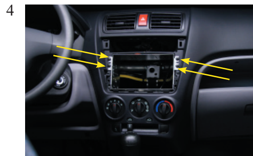
Place the 2-Din metal bracket and tighten it by four screws.
