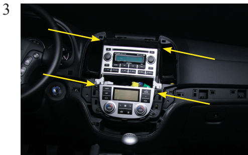
Remove the original radio. This is tighten by screws at the location of the arrows.
