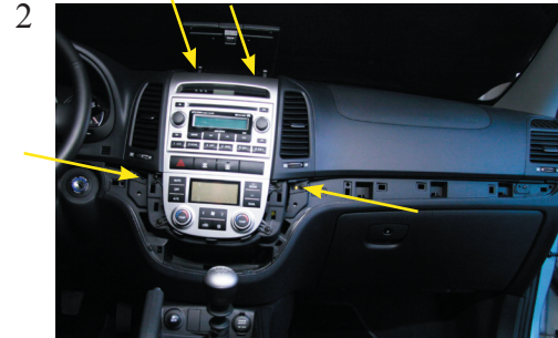
Remove two screws at the location of the arrows. These are in the storage pocket. Remove the air ventilation shafts. This is tighten by screws at the location of the arrows.
