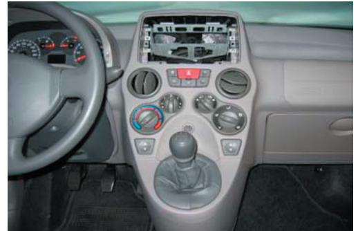
Remove the radio using Philips/ Blaupunkt radio keys.
