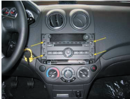
Remove the four screws at the location of the arrows.
