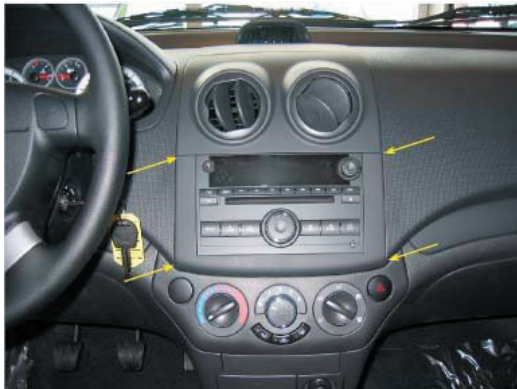
Use a plastic wig to loosen the panel.
