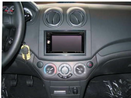
Place the head unit and connect all the wiring.
