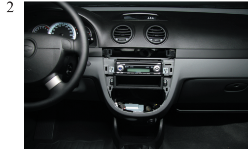
Remove the radio and the storage bin. This is tightened by screws.
