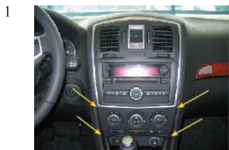
Use a plastic wig to loosen the panel at the location of the arrows.
