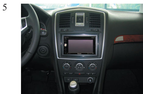
Place the headunit and connect all the wiring. Gently replace all the panels in reverse order.
