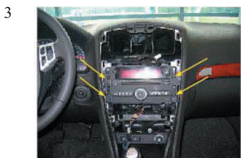
Loosen the screws at the location of the arrows. Remove the original radio.
