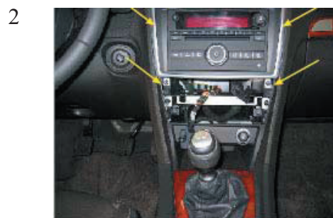
Remove the two screws at the location of the arrows. Now you can gently remove the panel.
