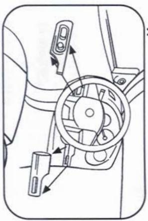
**6** Unclip and remove side panel from passenger side of dash with door open and remove (2) 7 MM screws from behind panel. (**Figure E**)
