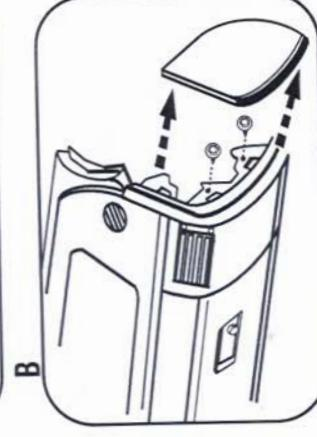
4 Unclip and remove side panel from passenger side of dash with door open and remove (2) 7 MM screws from behind panel. (Figure B)
