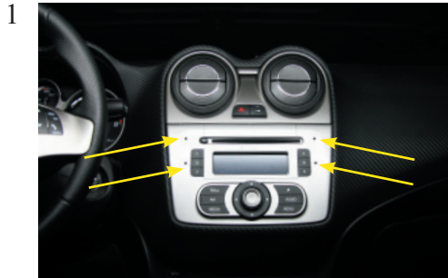
Remove the original radio using Philips radio removal keys.
