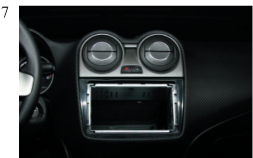
Place the 2-din metal bracket.
