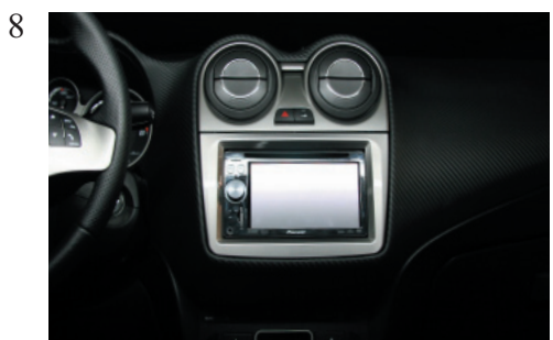
Place the headunit. Place the replacement panel.
