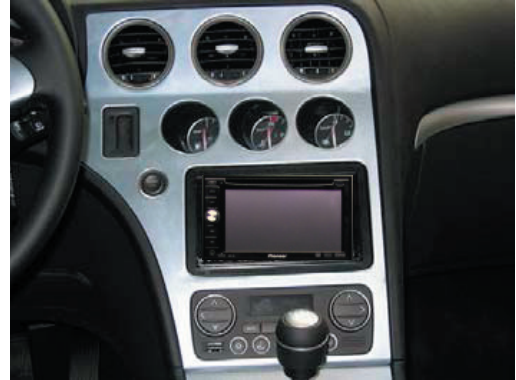
Place back all panels in reverse order. Place head unit and place rim.
