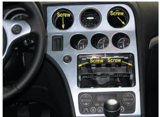
Remove 4 screws at the location of the arrows.
