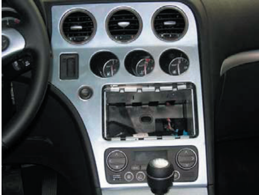
Place dashboard panel back en mount metal bracket. Connect all wiring.
