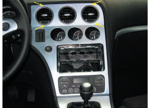
Remove 2 outside air ventilation shafts using a wedge. Start at the location of the arrows.
