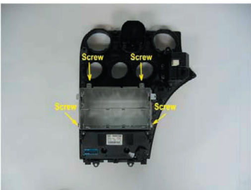
Remove original metal bracket from dashboard. Remove 4 screws at the location of the arrows.
