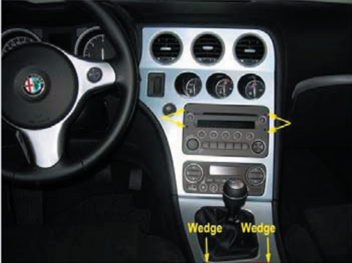
Remove radio using radio removal keys. Remove plastic cover around gearlever. Use wedge and start at the location of the arrows with wedge.
