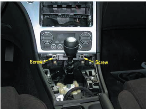
Remove 2 screws at the location of the arrows.
