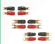
MC5-5F fork connector for 5 sq.mm cable, with 5 mm connection hole MC5-10F fork connector for 10 sq.mm cable, with 5 mm connection hole MC5-20F fork connector for 20 sq.mm cable, with 5 mm connection hole MC8-20F fork connector for 20 sq.mm cable, with 8 mm connection hole MC8-5R eyelet connector for 5 sq.mm cable, with 8 mm connection hole MC8-10R eyelet connector for 10 sq.mm cable, with 8 mm connection hole MC8-20R eyelet connector for 20
