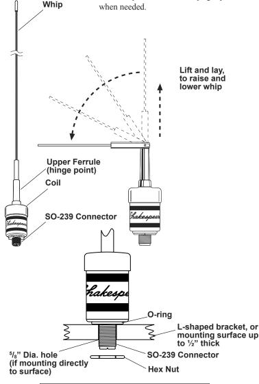
Tech Tip: This antenna will read "open circuit" when tested with an ohm meter or continuity tester.
