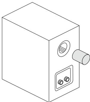
*To rightly tune the sound of Musa 105 with the acoustics of your ambience, it is possible to reduce the bass frequencies level, simply fitting the supplied foam plug in the reflex vent: usually when the speaker is placed inside a niche.*
