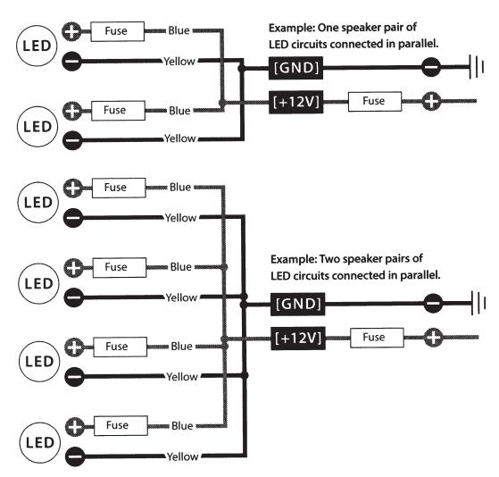
Individually fuse each BLUE (+12V) lead and wire together (parallel) to a fused, switched +12V activation circuit.
