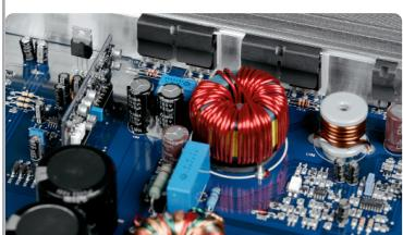
**Special steel springs** are used to fix the power transistors, providing superior heat transfer from the device to the heatsink. The special split design provides precise pressure on each device, avoiding potential thermal issues caused by poor contact between the devices and the heatsink. Thanks to this detail, the thermal efficiency is increased, allowing the power devices to work with lower average temperatures.
